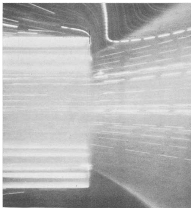
Fig. 5. Velocity field of viscoelastic fluid, q = 21.75 gal./min.
